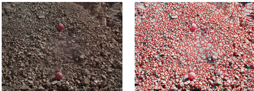
Fig. 6. A densely packed particle image from a rockpile (USA). Image resolution is 512x512.
